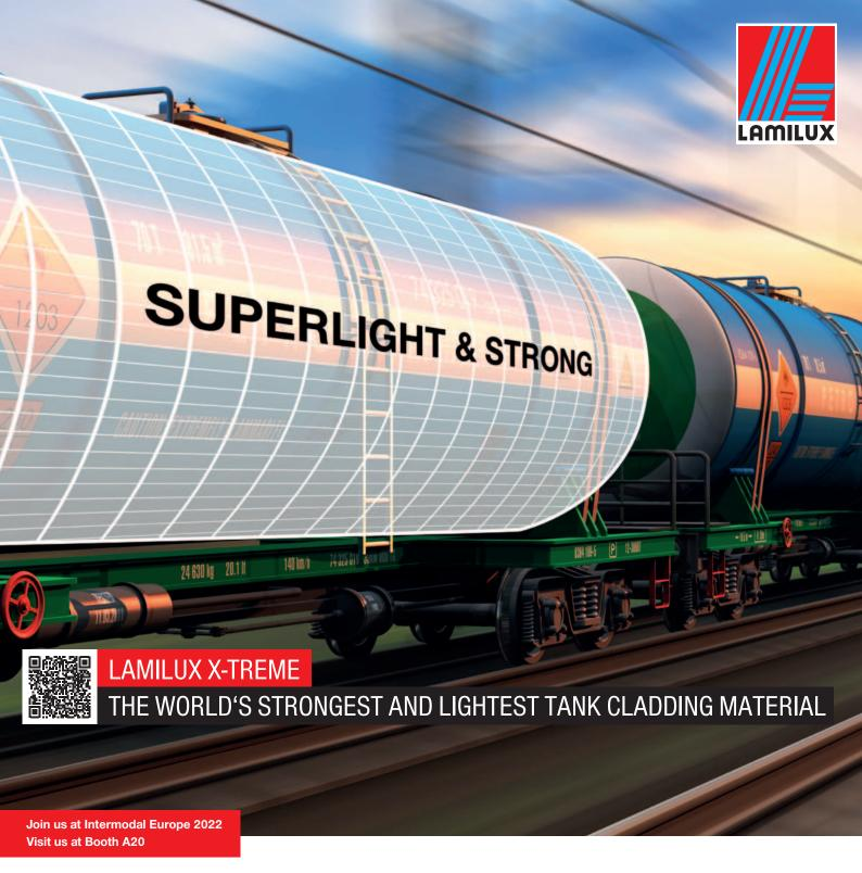
LAMILUX X-treme is the state of the art GRP material for tank claddings. It is a fiber reinforced composite offering the maximum possible content of reinforcement fibres in a highly elastic epoxy resin matrix. Highest strengths (twice than steel), outstanding impact tolerance and maximum weight saving can be are achieved. LAMILUX X-treme has three times the strength of the best tank cladding materials available in the market.
