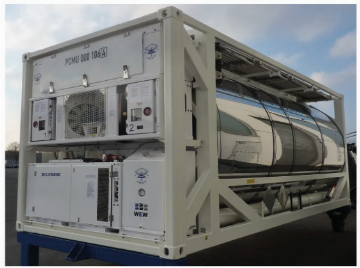
Dual Refrigeration System for Tank Containers
