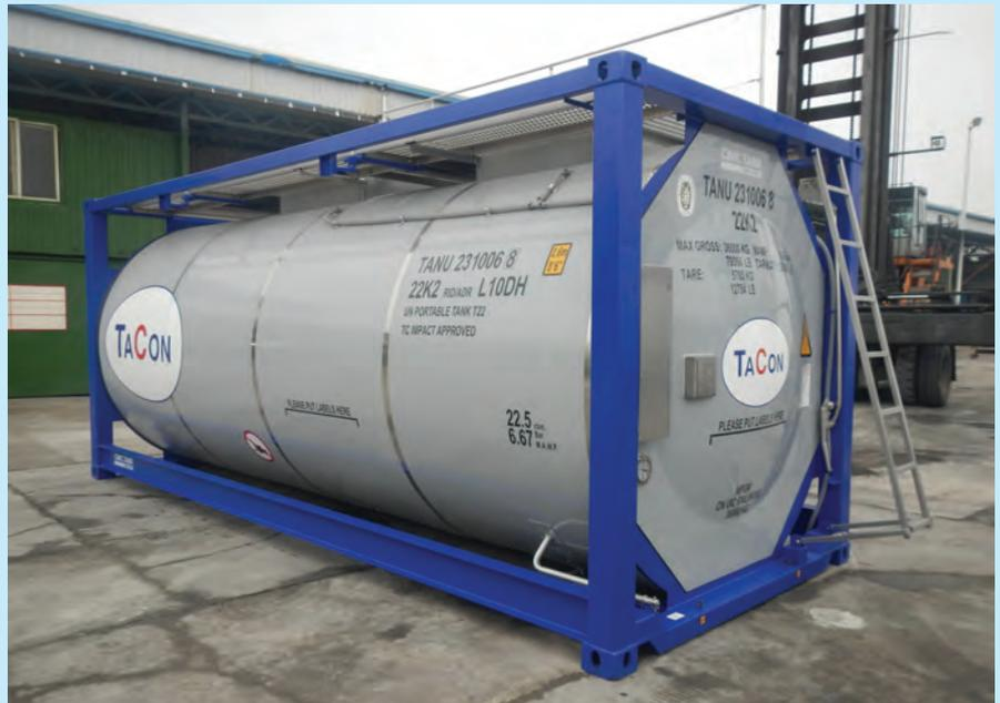
are available with or without electrical heating system for temperature sensitive products.
