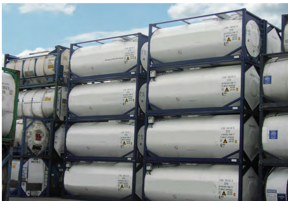
Container Safety Convention (CSC) certification includes stacking ratings as well as racking, lifting and stacking tests
