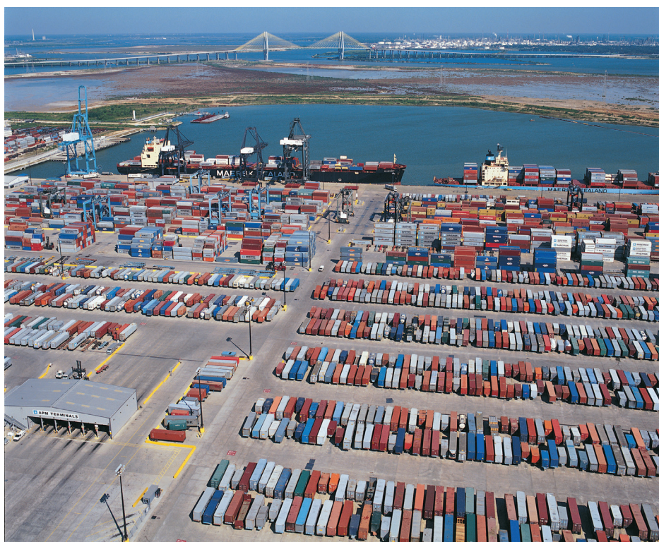
The port of Houston will improve operational efficiency by switching from chassis to ground storage served by RTG cranes
